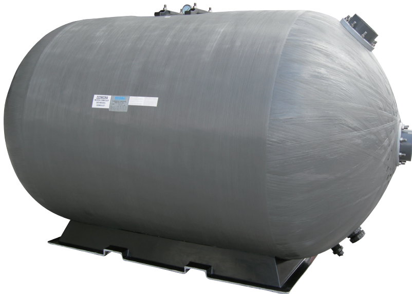
Waterco’s Micron Commercial fibreglass filters are made from continuous strands of high quality fibreglass filament wound under controlled tension to create a seamless, impervious vessel. This produces a filter that is free from welds or seams, or special tank linings that typically corrode or electrolyse.
