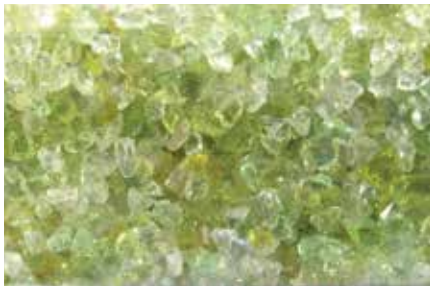
Ecopure glass has undergone specialised heat treatment process, which reduces degradation and therefore lengthens its life span.
